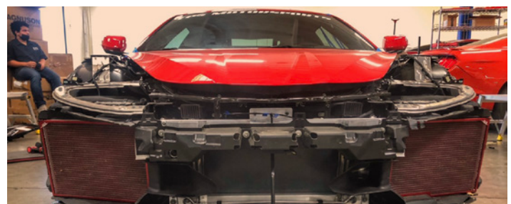
C8 Corvette with front fenders, bumper, & lights removed for Lambo Door Install. TPS C8 Radiator Screens installed
